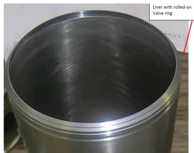
Fig. 15 Liner with rolled-on valve ring
